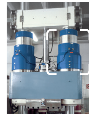
Hydroforming press Generating 400 metric tons closing force
