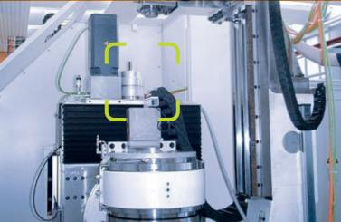
Securing the Z-axis in case of emergency stop and for maintenance
